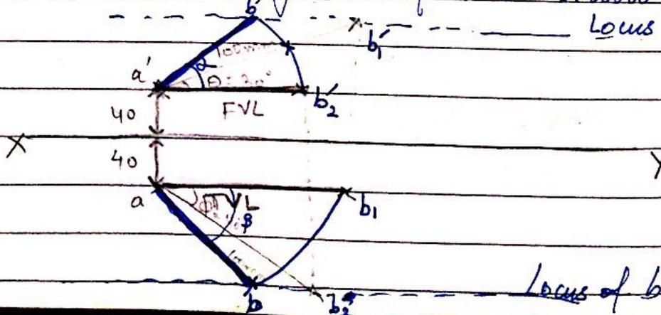
eg 3) The end pt. A of a line AB is 30 mm in front of VP & 50 mm above HP. The line is inclined at  $40^\circ$  to HP & FV is  $50^\circ$  to XY. The TV is 120 mm long. Draw its proj<sup>n</sup>.
