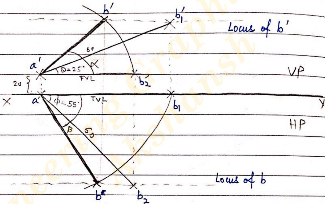
Q A line ~~AB~~ <sup>AB</sup> 90 mm long measures 72 mm in FV & 65 mm in TV. Draw 2 views of the line. Fully in 1st quadrant. Find true inclin<sup>n</sup> of the line. Assume a pt. A ~~at~~ at a suitable distance from resp. planes.
